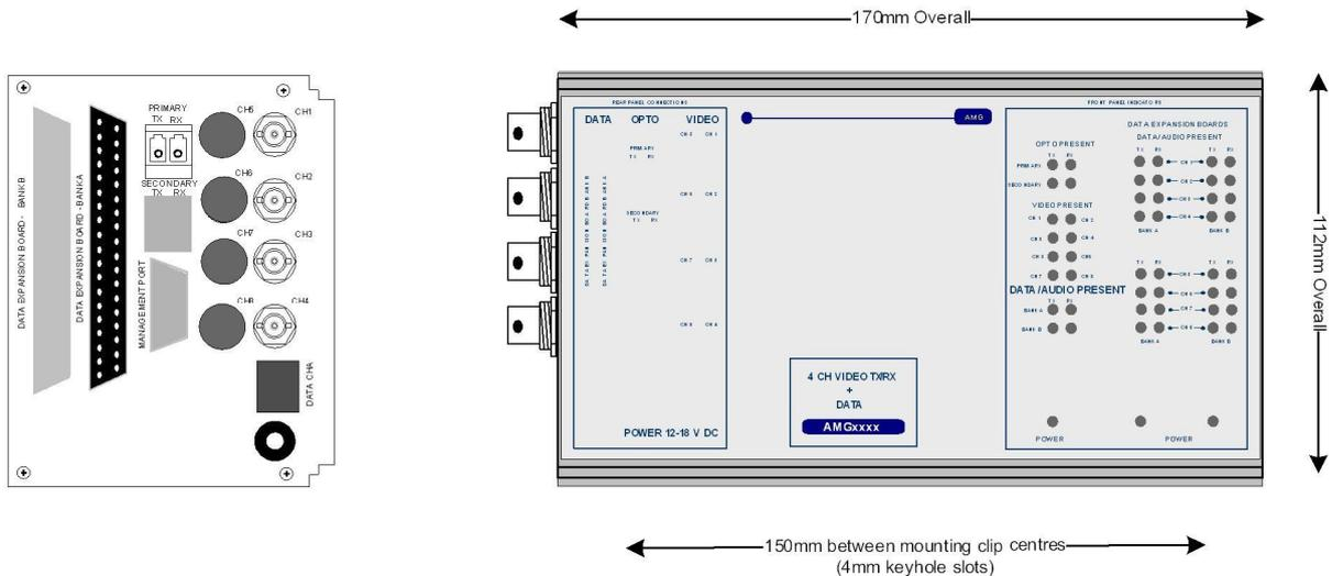
The **AMG4647A-SF** is a standalone four channel video transmit unit designed to transmit 4 video signals and transmit and receive up to 8 data or audio signals over one Multimode fibre. The 8 data/audio channel interfaces, whether RS232, RS422, RS485, 20mA, TTL, Contact Closure, Lonworks or Audio, are defined at manufacture by the addition of daughter boards fitted onto the Data Expansion Board A.
